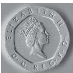
Fine surface structures provided by photometric stereo
